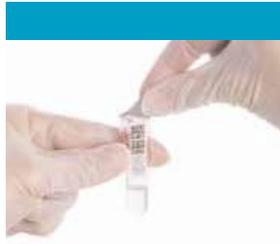
**1** Remove the foil cover from the cuvette. The liquid surface should lie between the two lines marked on the cuvette. Do not touch the clear flat surfaces in the lower part of the cuvette.
