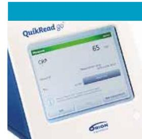
**7** When the measurement is completed, the result is shown on the display and the cuvette will rise up from the measurement well automatically. With the QuikRead go wrCRP+Hb test the Hb result is shown below the CRP result.
