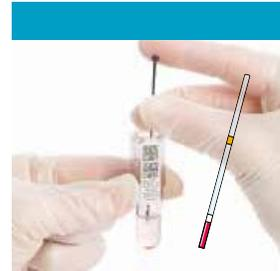
**3** Place the sample (10 µl) into the buffer solution in the cuvette and dispense by pressing down the plunger. Make sure that the capillary is completely empty.
