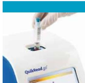
**6** Insert the cuvette in to the measurement well of the instrument. The bar code should be facing you. The display shows how the measurement is proceeding.
